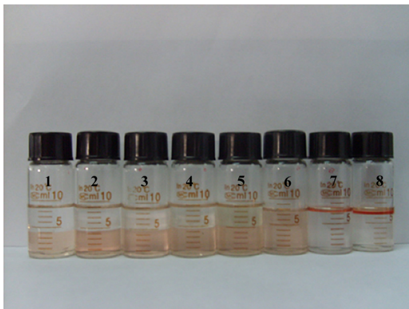
Fig. 2. Extraction of Cyt-c employed PEG and IL /potassium citrate systems at 30 °C. 1: PEG1000 (18%, w/w)/potassium citrate (20%, w/w); 2: PEG2000 (18%, w/w)/potassium citrate (20%, w/w); 3: PEG4000 (18%, w/w)/potassium citrate (20%, w/w); 4: PEG6000 (18%, w/w)/potassium citrate (20%, w/w); 5: PEG10000 (18%, w/w)/potassium citrate (20%, w/w); 6: [C 2 mim]Br (6.25%, w/w)/potassium citrate (41.7%, w/w), no phase separation; 7: [C 4 mim]Br (6.25%, w/w)/potassium citrate (41.7%, w/w); 8: [C 6 mim]Br (6.25%, w/w)/potassium citrate (41.7%, w/w). [Cyt-c] = 20 µg/g.
